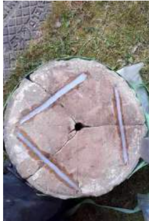
Slots being ground into the urn and afterwards with the flat-bar set-in with the now hard, external grade epoxy-resin.
