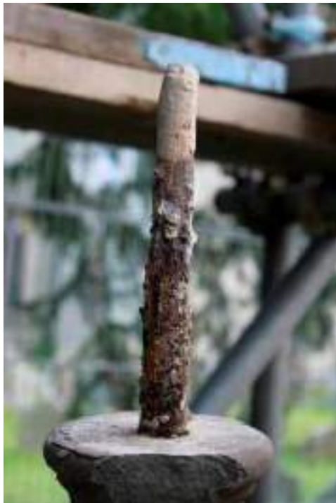
On the left, after removal of the fractured lower section, see how the delaminating iron-dowel had expanded into the available space before forcing the stone apart, exerting huge pressure to split the block. On the right, the repaired lower urn section with new, threaded stainless-steel dowel issuing from the top. The drill-hole between the steel (which cannot corrode) was filled with a pourable anchor grout used in civil engineering.
