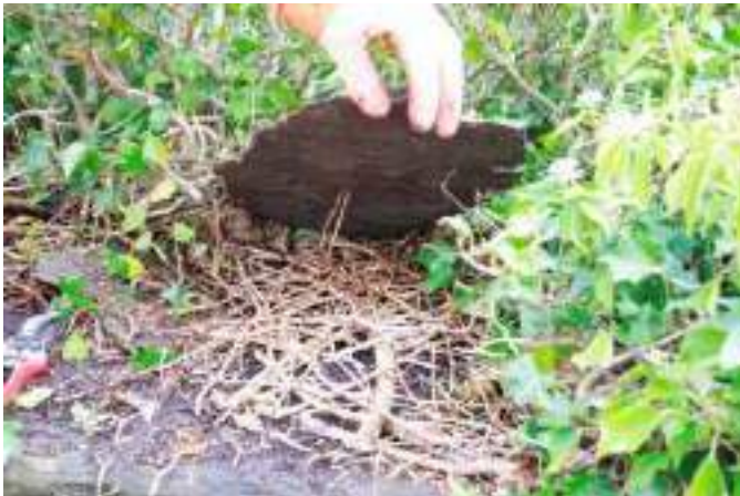
The ivy tendrils had exploited the laminations of this weak laminar stone, growing along bedding planes and forcing layers apart.
